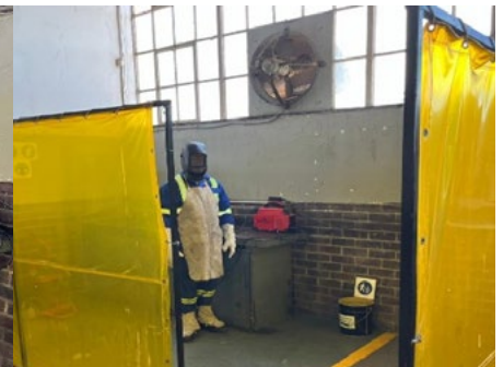
Appropriate PPE (personal protective equipment) for welding worn. Welding Screens being used to prevent workers operating in close vicinity of the welding area are not exposed to harmful UV light or the risk of flash burns.
